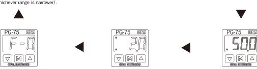
Press (M) button once. Both SW1 and SW2 LEDs will turn off and the Digital filter setting will be displayed. Set the value in the same manner. Response time: (F-0, 1, 2, 3, 4): (2.5, 250, 1000, 2000) ms F-0 (2.5ms) is set prior to delivery.
